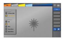
Invisible light source (1310 or 1550ns) can provide the following types of light, including CW light, 1kHz light, 2kHz light, 1kHz blink light, 2kHz blink light.
